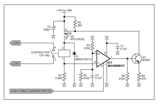
Figure 1. This contactor circuit self-oscillates to minimize power consumption when on.
